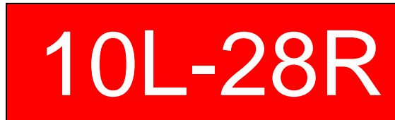
Runway Hold Sign
