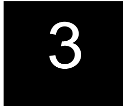
Runway Distance Remaining Sign
