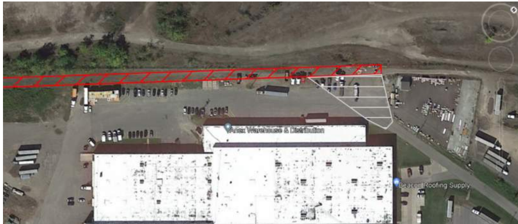
Potential Haul Road (Red Hatch) and Lot Improvements/Restrictions (Gray Hatch)
