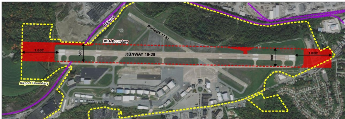
Figure 1-3 Runway 10-28 Standard RSA Deficit (red)
